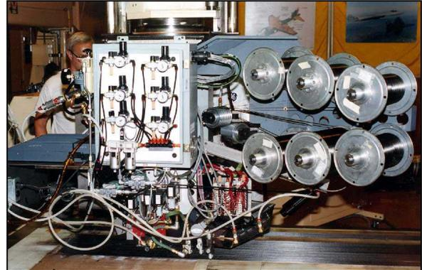
Figure 1 In-situ deposition head consolidating 12 IM-7/PEEK tows on a laminate up to 5mpm (20fpm)
