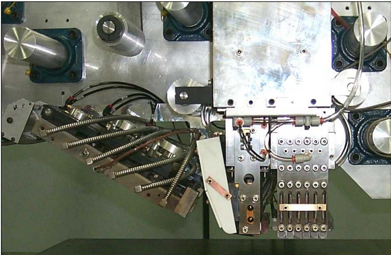
Figure 3 The hot line and the hot area compactors are integrated together with a feeder on an evaluation frame so that their conformability can be evaluated while placing composite tape.
