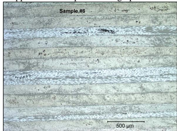
Figure 24 Photomicrograph of the laminate in the 45° crease region #6 between the top and side ramps.
