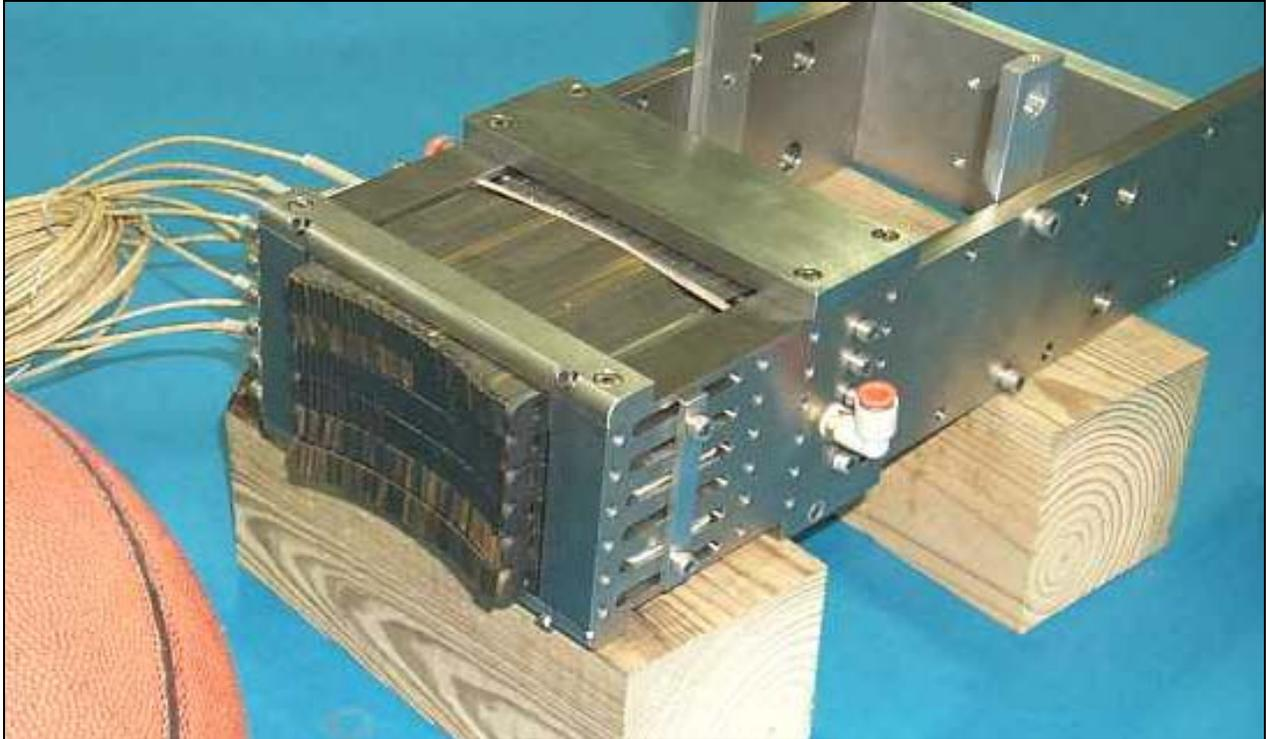
Figure 6 Hot area compactor's conformance to a basketball. The compactor pushes with a 400N (100-lb.) force at 450°C over a 114mm by 76mm area (4.5-in by 4-in).
