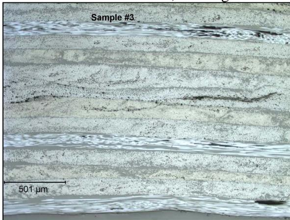
Figure 21 Photomicrograph of the laminate in the transition region #3 between the ramp and the upper land.
