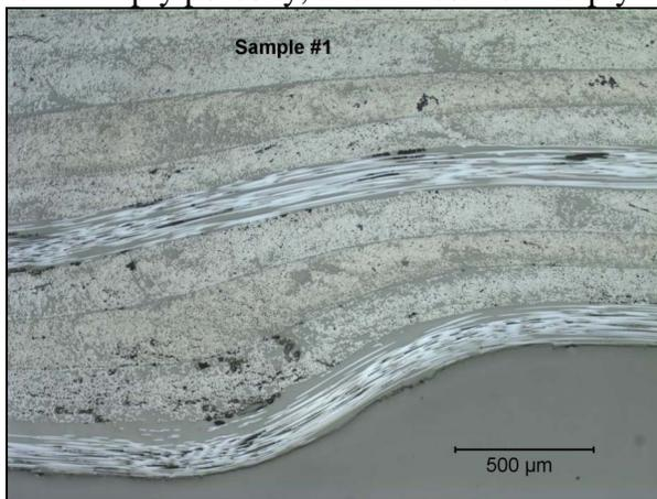
Figure 19 Photomicrograph of the laminate in the transition region #1 between the lower outside flange and the ramp.
