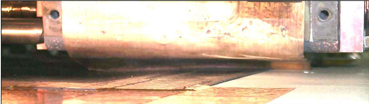
Figure 8 The hot line compactor conforms to the pan-down tool while laying PEEK tape.
