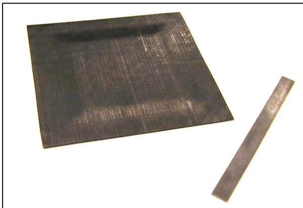
Figure 12 Top surface of [0/-45/90/45]<sub>2s</sub> pad-up laminate produced on pyramid shaped tool
