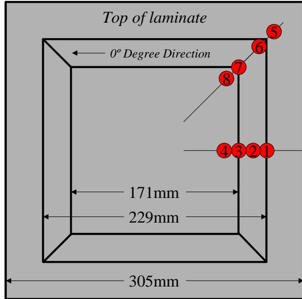
Figure 18. Laminate dimensions for the 16 ply  $[0/-45/90/45]_2s$  IM-7/PEKK laminate. The numbered circles indicate the locations where photomicrographs were taken.
