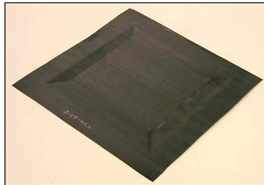
Figure 9 The completed IM-7/PEEK pan-down laminate, with a  $[0/90/0/90]_s$  laminate stacking sequence
