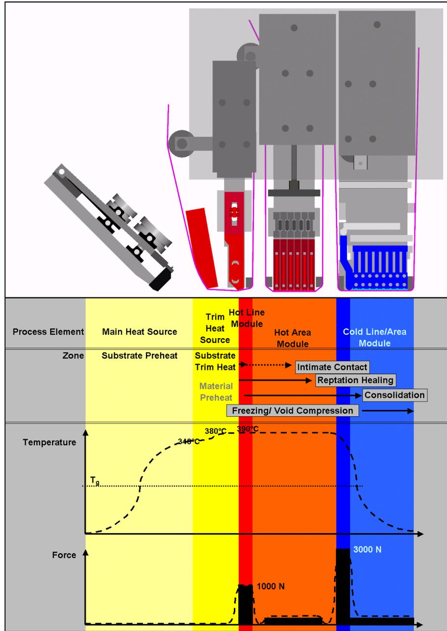
Figure 2 Fiber placement process zones and process parameters
