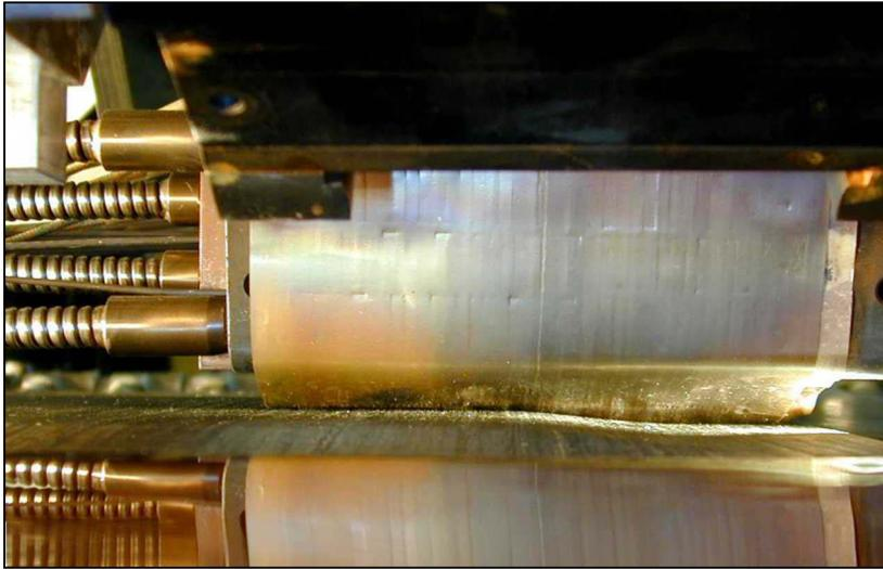
The head is placing in the 0° direction in the figure. Figures 15 and 16 show the head placing in a 45°-course direction over the center of the laminate, where two ramps come together to form a 45°-crease. In Figure 16, the shim was removed to reveal the shim conformance against the laminate from the back side.
