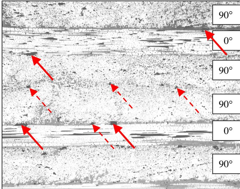
Figure 11 shows that the laminate quality in the ramp area is slightly worse than the quality in the center of the pan-down laminate. There are some very small interlaminar voids between the two center 90° plies. There are one small and two larger interlaminar voids between the lower-middle 90° ply and the 0° ply below it. There is also one void between the top-middle 90° ply and the 0° ply above it. The voids are labeled with arrows. The rest of the interfaces are well healed.
