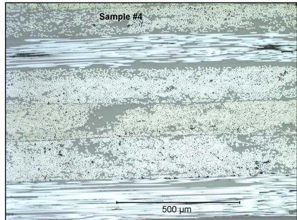
Figure 22 Photomicrograph of the laminate in the upper land region #4.
