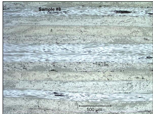
Figure 26 Photomicrograph of the laminate in the upper land region #8.
